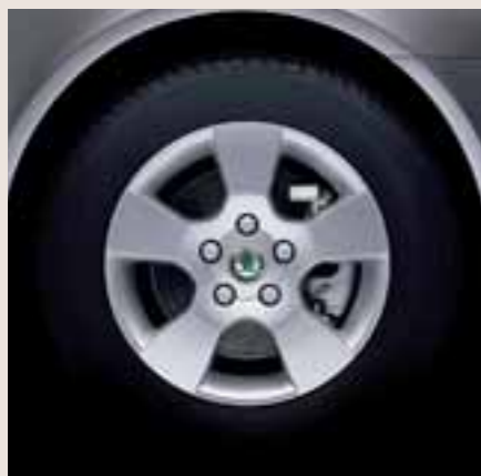
6.5J x 15" Helios alloy wheels with 205/60 R15 tyres. Standard equipment for the 4x4 Elegance version. Extra equipment for the Classic, Ambiente, Elegance and 4x4 versions.
