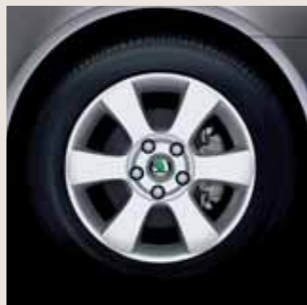
6.5J x 16" Lyra alloy wheels with 205/55 R16 tyres. Extra equipment for the Classic, Ambiente, Elegance, 4x4 and 4x4 Elegance versions.
