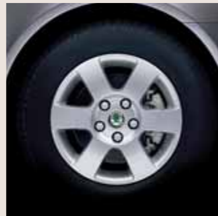
6.0J x 15" Orion alloy wheels with 195/65 R15 tyres. Standard equipment for the Elegance version.
